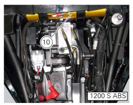
Undo the fixing screws (8) of the bracket (9) and remove the expansion reservoir (10) of its seat.
