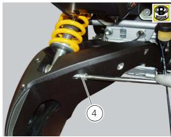
For 1200 ABS model position the adjusting knob (A) of the preload on the support bracket tightening the screws (19) to the specified torque (sec. 3 - 3, Frame torque settings).
