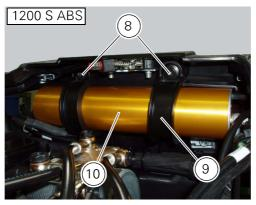
Connect the connector (B) of expansion reservoir (10) of the shock absorber to the main wiring.
