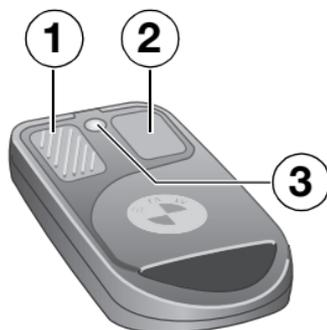
Synchronisation is necessary if the buttons on the remote control unit are pressed more than 256 times outside the range of the receiver. When this limit is reached the receiver on the motorcycle no longer reacts to signals from the remote control unit.
